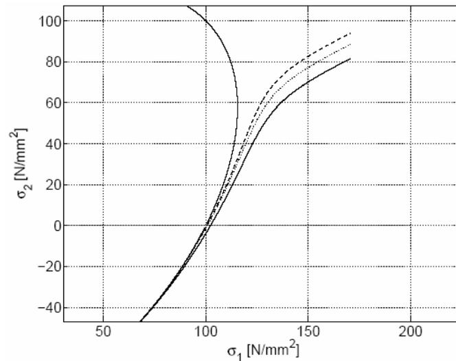
*Results of tests where the yield surface can be traced with the algorithm.*
